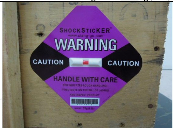
Photo "J" After testing - Purple 37g(L55)
