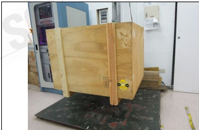
Photo "G" Drop test- -Yellow 25g(L65)
