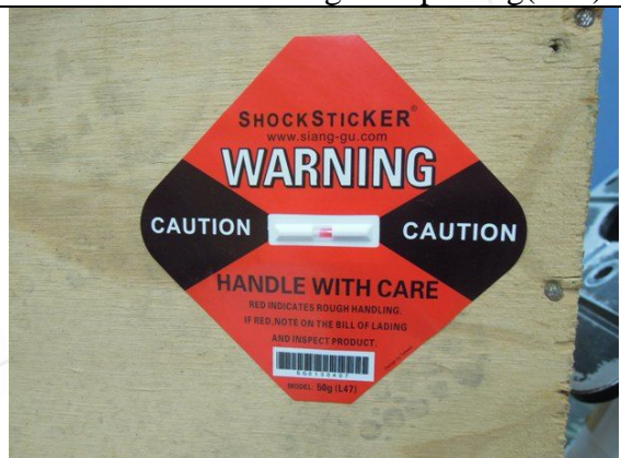
Photo "L" After testing - Red 50g(L47)
