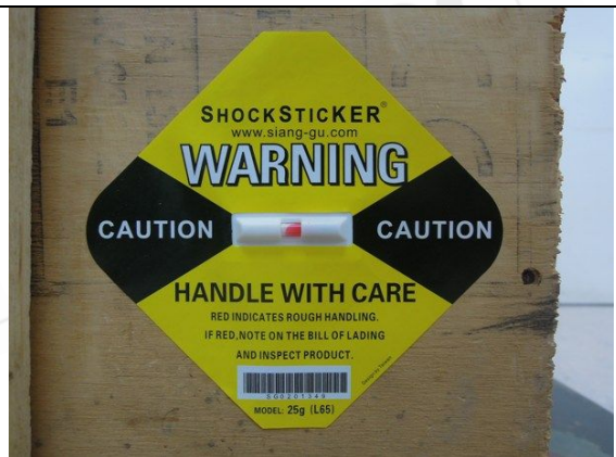
Photo "H" After testing - Yellow 25g(L65)
